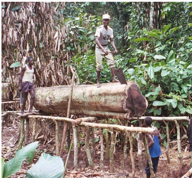
Figure 21. First cut on bokenge ( Hua gabonni ) log, 70 cm diameter x 3.9 m long, felled with axe. (Photo by Rick Alexander)
