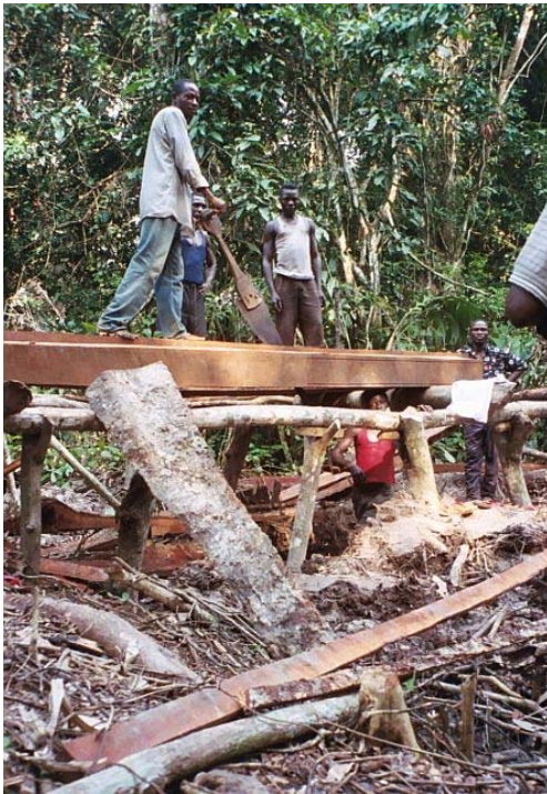
Figure 22. Longsaw operation. Trees are felled with axe and sawn into planks using long saw. (Photo by Rick Alexander)
