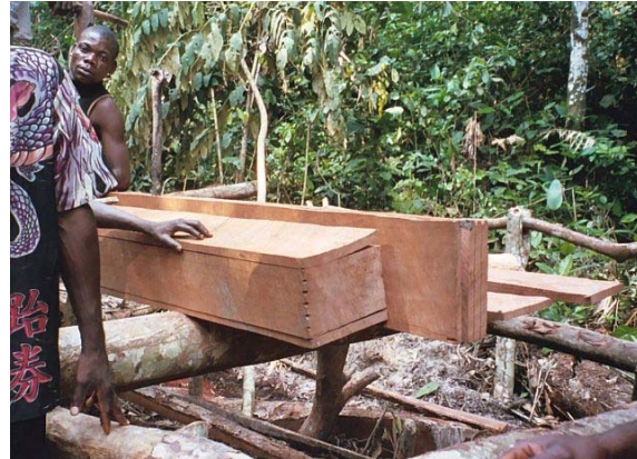
Figure 4. Rough cut log is marked and notched to guide sawing into planks. (Photo by Rick Alexander)
