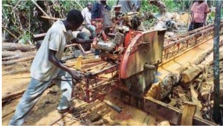
Figure 23. Mobile Dimension Saw operated by 5-person crew plus 5 people carrying planks to road 1 km away. (Photo by Rick Alexander)
