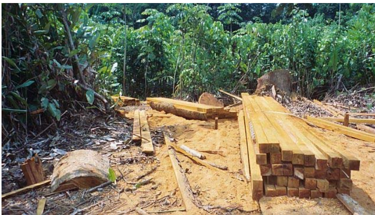
Figure 7. Planks cut by mobile power saw, 7x7cm x 5.2m. (Photo by Rick Alexander)
