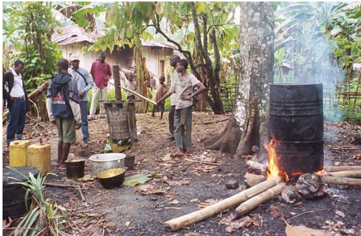
Figure 2. Palm oil processing operation; palm nuts boiling in drum on right, then pressed and stored in the 25-liter yellow jugs. (Photo by Rick Alexander)
